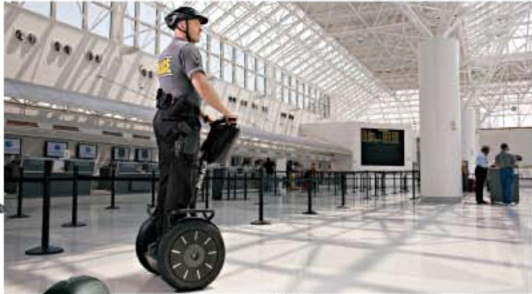
develops a maximum speed of 20km/h and can drive 39 kilometres on a single battery charge. It weighs just 50kg and the driver has no control commands. The acceleration, braking and turning is done only by the movements of the driver's body.
